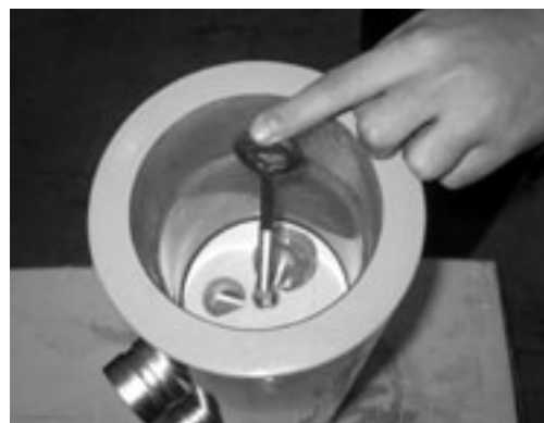
Figure 8.6 – Stand ceramic cartridge on blocks
