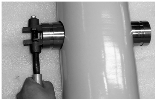
Figure 8.7 – Remove PX-140S side ports with inside wrench if removing center manifold
