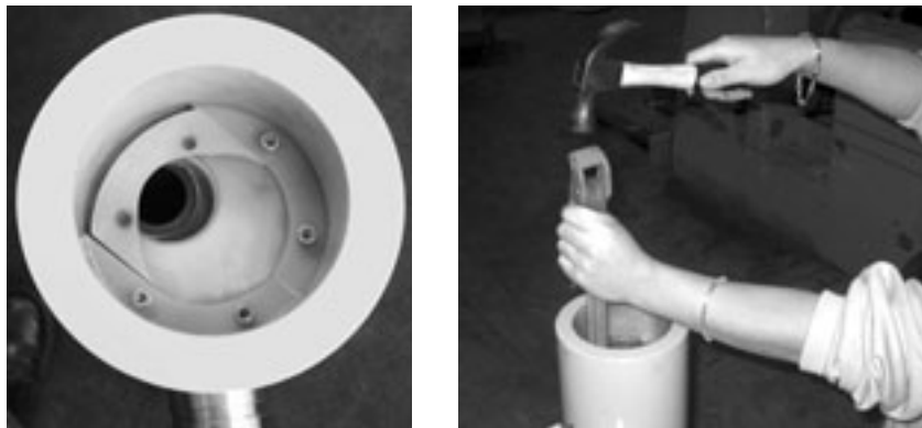
Figure 8.2 – Remove cap screws, locking rings and access cover from the end of unit. Tap down to loosen access cover if necessary.
