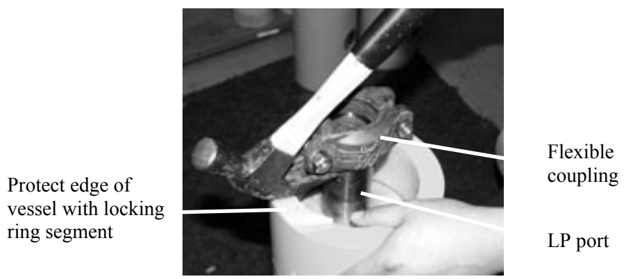
Figure 8.3 – Pry off access cover using LP port with flexible coupling
