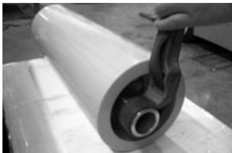
Figure 8.1 - Remove LP IN port from the end of unit
